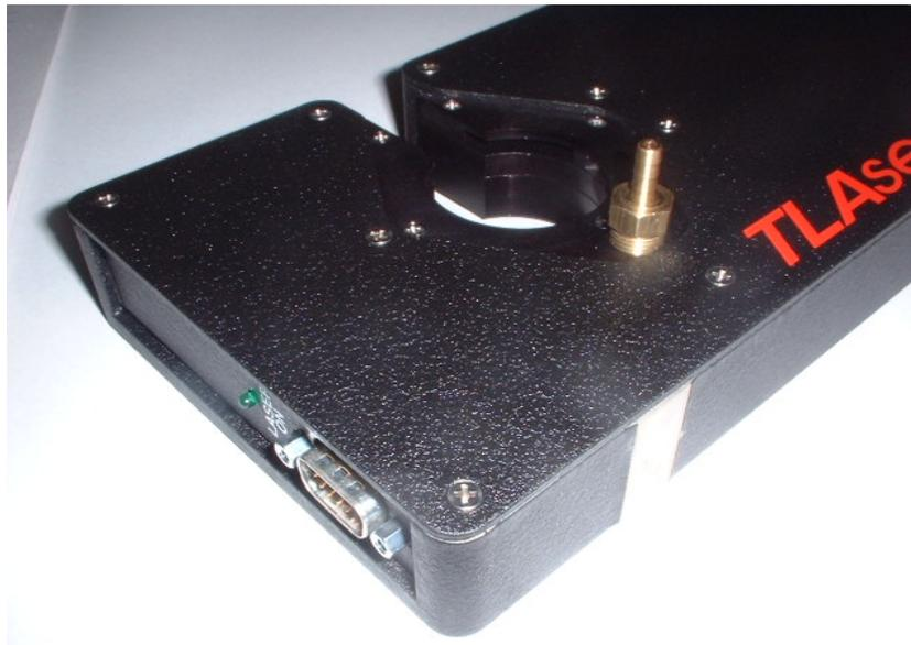
*TLAser222 with air purge installed.*
